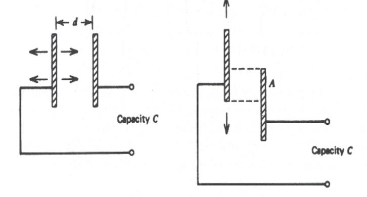
Capacity varies with the distance between the plates and the common area. Both effects are used in sensors.
